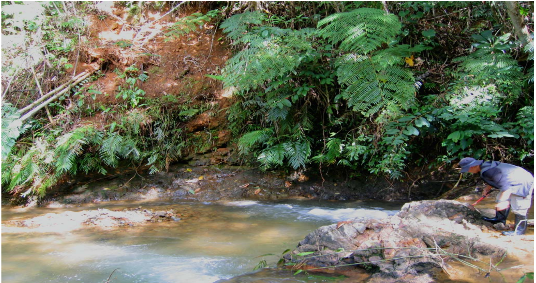
Plate 1. Photograph looking south-southeast showing the thrust contact with unmineralised quartz diorite on the right and reddish sheared basaltic rocks on the left. The sharp thrust contact dipping approximately 65^\circ to the east is immediately in front of sampler.
